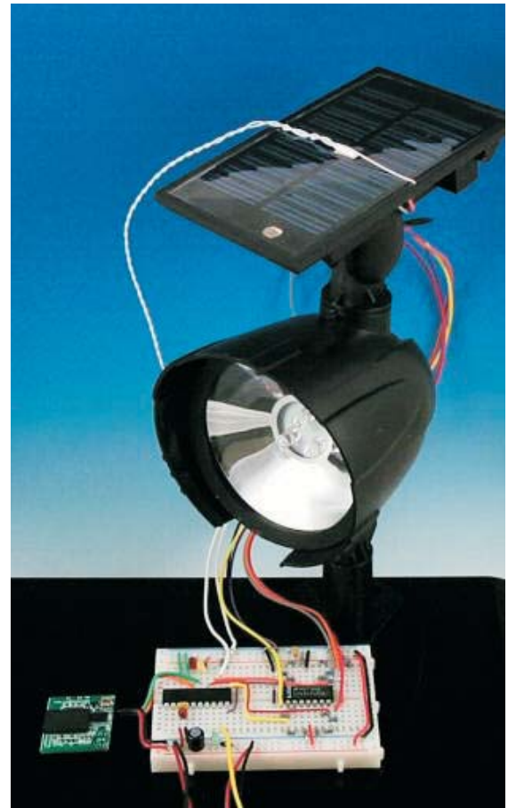
Figure 1: Hampton Bay Solar LED Spotlight with LabRecon chip and circuitry on solderless breadboard
