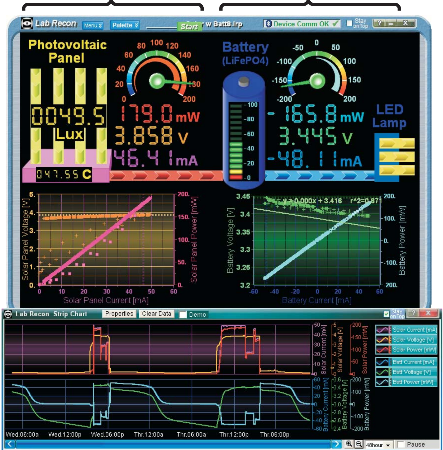
Figure 3: LabRecon screen shot including strip chart view of 48 hour time span
